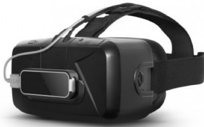
Fig. 5. Oculus Rift VR headset and mounted Leap Motion controller for hand tracking.
