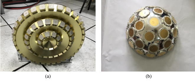
Fig. 7. Irregular antenna arrays for space/air/ground communications. (a) triple round phased arrays in X-band, (b) hemisphere antenna array in S-band.
