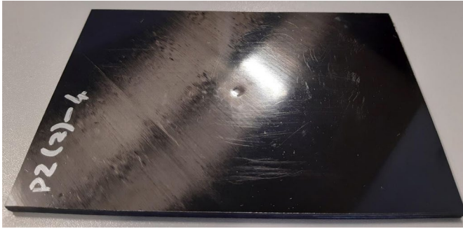
Fig. 2 Photograph of a CF/Epoxy composite panel 150 mm x 100 mm in size with a thickness of 4.6 mm after an impact of 7.5 J showing a typical surface indentation
