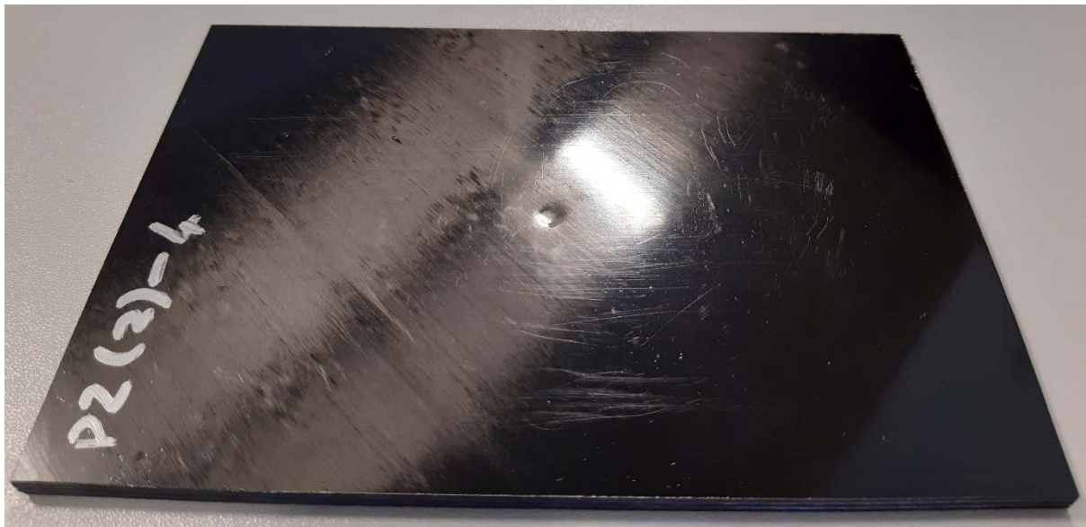
Figure 2. Photograph of a CF/Epoxy composite panel 150 mm x 100 mm in size with a thickness of 4.6 mm after an impact of 7.5 J showing a typical surface indentation.
