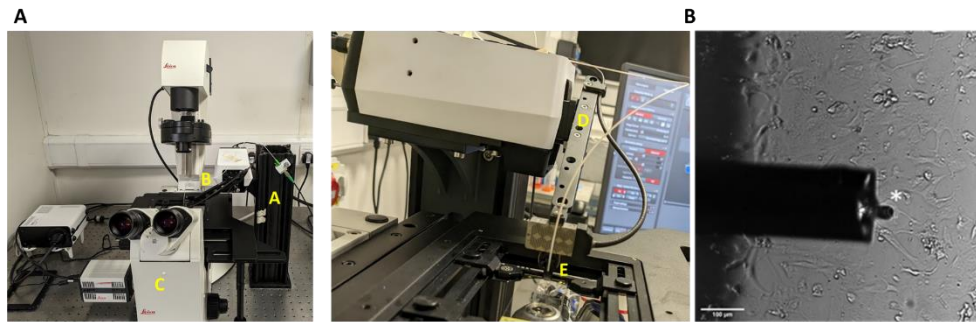
Figure 2.3: Overview of the Chiaro Piuma nanoindenter set-up A) Set-up of the nanoindenter. (Yellow text) A) The nanoindenter body, B) The arm of the nanoindenter, C) Leica DMI8 Epifluorescence, D) closer, and alternative view showing nanoindenter arm, E) Probe tip. Using an inverted Leica DMI8 microscope the nanoindenter was situated to the right. The arm of the nanoindenter with the probe attached was lowered over the 10x or 20x objective lens. B) Brightfield image showing the nanoindenter probe (spring constant, 0.49 N/m; radius, 49 \mu\text{m} ) at 20x zoom highlighted by the asterisk. Scale bar= 100 \mu\text{m} .
