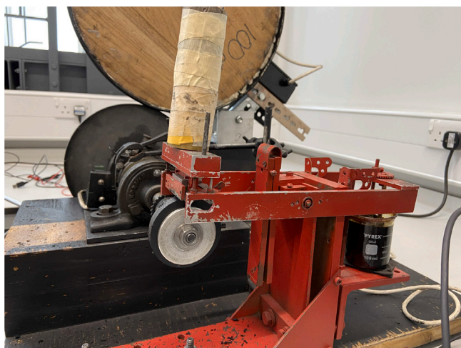
Fig. 1. Blade abrasion machine used for the production of smear wear particles.
