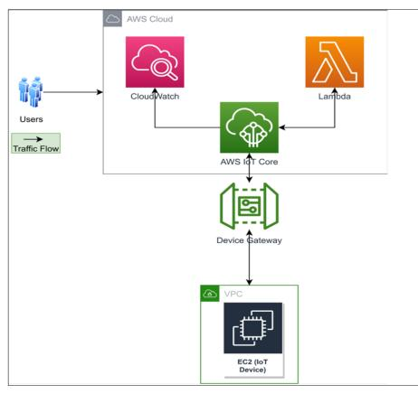
Figure 4. IoT system architecture implementation using AWS-1-.
