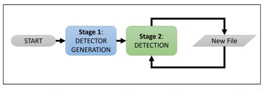
**Figure 1.** Stages for detector generation and detection in artificial immune systems. The new file represents incoming files which may be benign or malicious.
