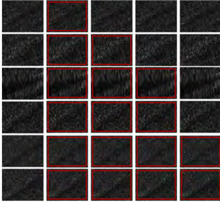
Fig. 15. Some examples for the ship wake detection results. The first column is the original image patches from SSDD, and the second, third, fourth and final columns respectively show the results of the modified AdaBoost, AdaBoost, Radon with GMC and Radon; the correctly detected patches are labeled with red box.
