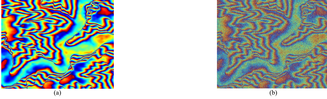
Fig. 4. The true interferogram and the single polarimetric noisy interferogram formed by the two simulated SLC images: (a) true interferogram; (b) single polarimetric noisy interferogram.
