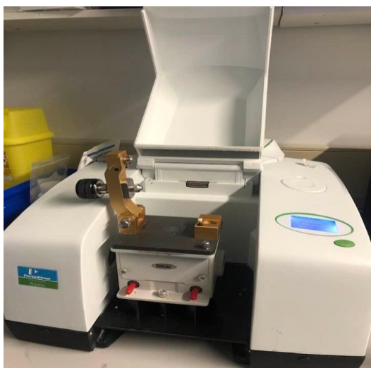
Figure 17 – FTIR analysis using the Spectrum GX (Perkin-Elmer, Waltham, MA, USA)
