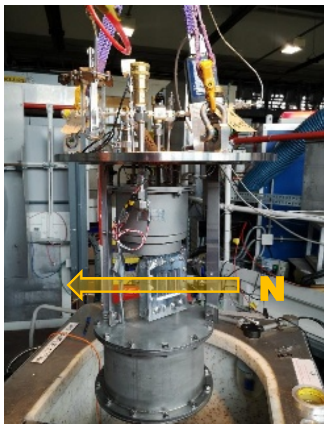
Figure 4 The CO 2 -mineralization reactor rig being installed into the sample area of the IRIS beamline at RAL-ISIS. The rig position is adjusted such that the neutron test cell is perpendicular to the incident neutron beam (N)
