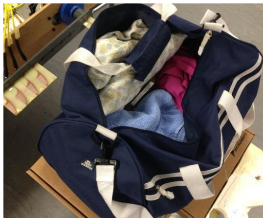
Figure 5-43 Experimental set-up of one metallic target in a stuffed sports bag
