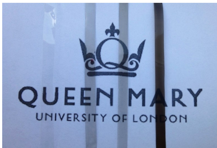
Figure 5.5: Picture of PVA nanocomposite strips. From left to right; neat PVA, PVA-GO 0.05 wt.%, PVA-GO 0.1 wt.% and PVA-GO 0.5 wt.%.
