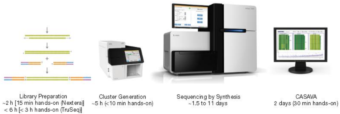
Figure 2.8 Illumina Hi-Seq 2000 platform. After library preparation, the fragments were amplified to create clusters, each containing ~1000 copies of the same template. The samples were then sequenced using SBS (sequencing by synthesis) technology. Figure adapted from Illumina website.
