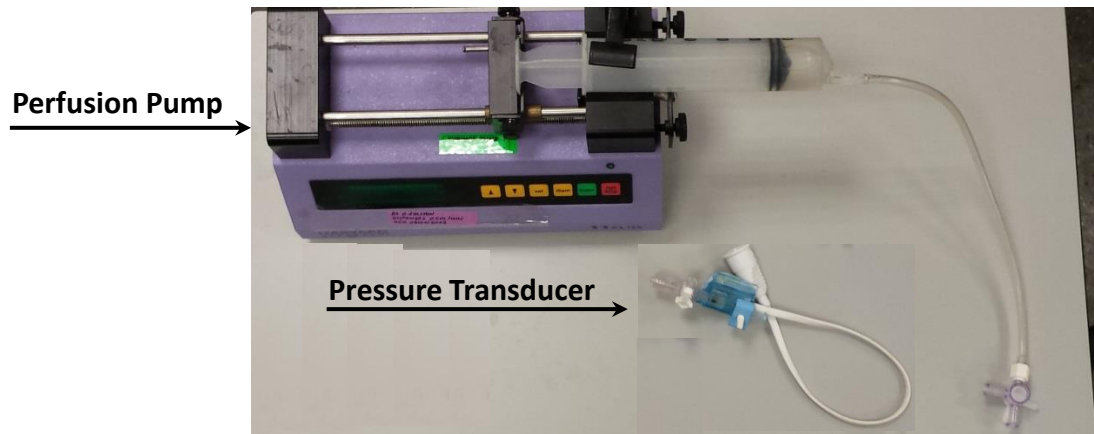
Figure 2.15: A perfusion pump and pressure transducer were used to lumenally distend appendices.
