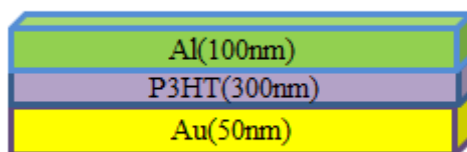
Figure 69: Schematic of an Au(50 nm)/P3HT(300 nm)/Al(100 nm) device.
