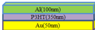
Figure 77: Schematic of an Au(50 nm)/P3HT(350 nm)/Al(100 nm) device.
