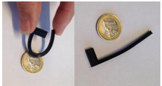
Fig. 27. 3D printed flexible antenna enabled by LM [178].
