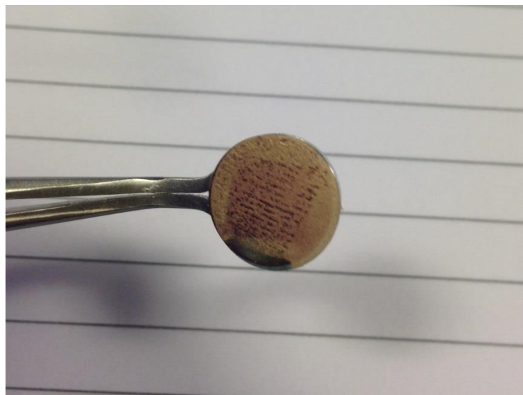
Figure 5.7 Degraded PLGA-PEGDA-DTT film
