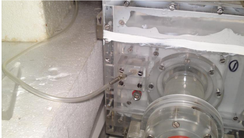
Figure 21: Small and large flow systems enter the proximal EVAR phantom housing
