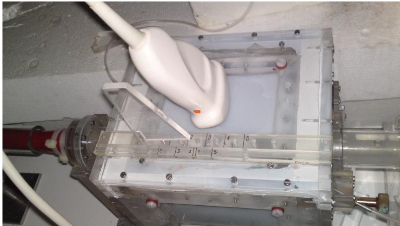
Figure 26: Curvilinear (2-5 MHz) ultrasound probe placed by positional jig, viewing the EVAR phantom and endoleak via the ultrasound viewing window
