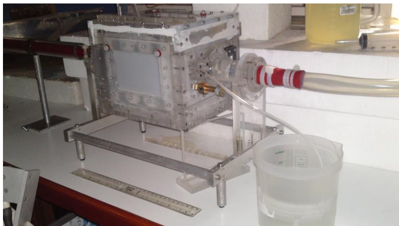
Figure 25: Distal aspect of the phantom showing the large and small flow systems exiting the housing
