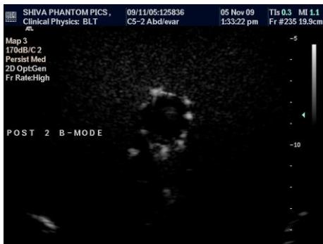
Figure 51: Images of the phantom simulated endoleak in a posterior position 2, using B mode, colour Doppler and contrast enhanced ultrasound
