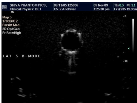
Figure 49: Images of the phantom simulated endoleak in a lateral position 5, using B mode, colour Doppler and contrast enhanced ultrasound
