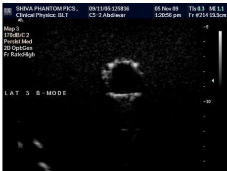
Figure 47: Images of the phantom simulated endoleak in a lateral position 3, using B mode, colour Doppler and contrast enhanced ultrasound
