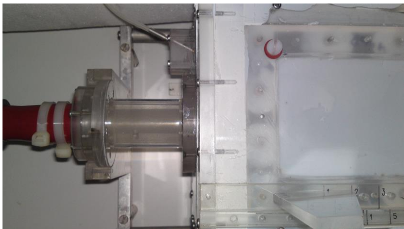
Figure 22: Superior view of small and large flow systems entering the proximal EVAR phantom housing
