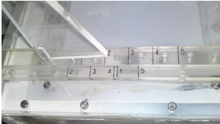
Figure 15: Viewing jig on the EVAR phantom ultrasound window: the probe can be placed at set positions standardizing images between subjects
