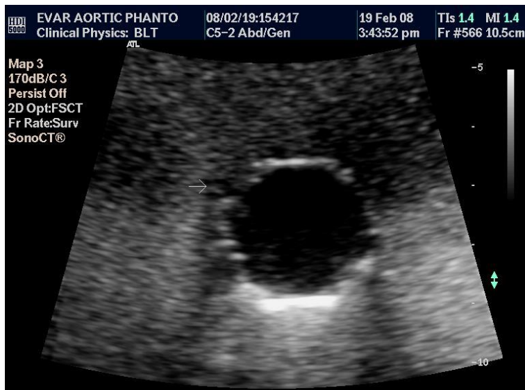
Figure 34: Transverse ultrasound B-mode image produced of the EVAR stent (large flow system) within the EVAR phantom
