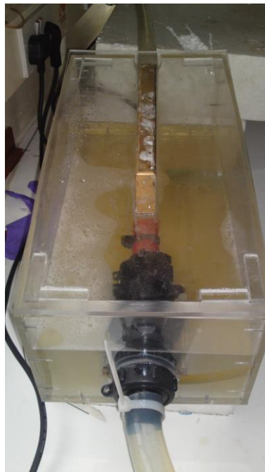
Figure 10: Doppler blood-mimic reservoir of the large (EVAR stent) flow system
