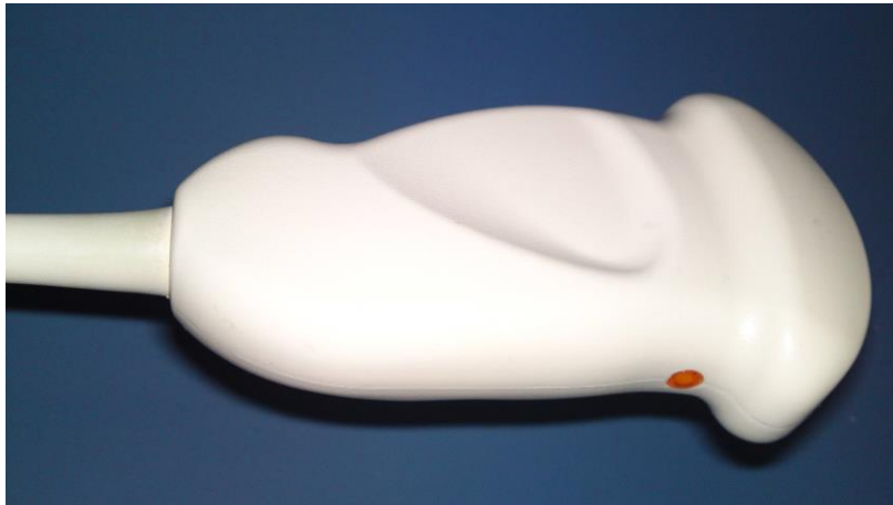
Figure 33: Phillips HDI 5000 ultrasound machine curvilinear probe used for the EVAR phantom experiments
