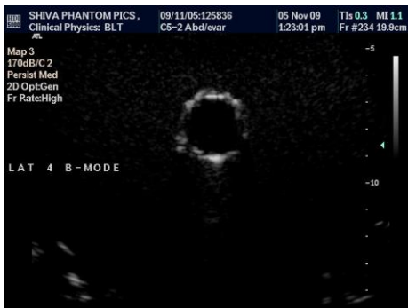
Figure 48: Images of the phantom simulated endoleak in a lateral position 4, using B mode, colour Doppler and contrast enhanced ultrasound
