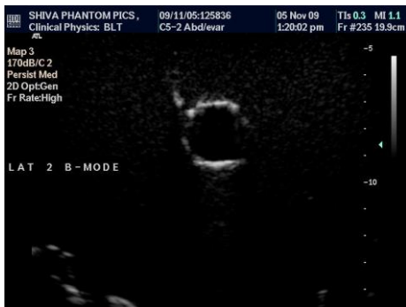
Figure 46: Images of the phantom simulated endoleak in a lateral position 2, using B mode, colour Doppler and contrast enhanced ultrasound
