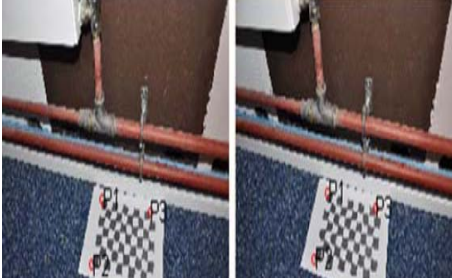
Figure 3.27: Non collinear points selected in pipe
