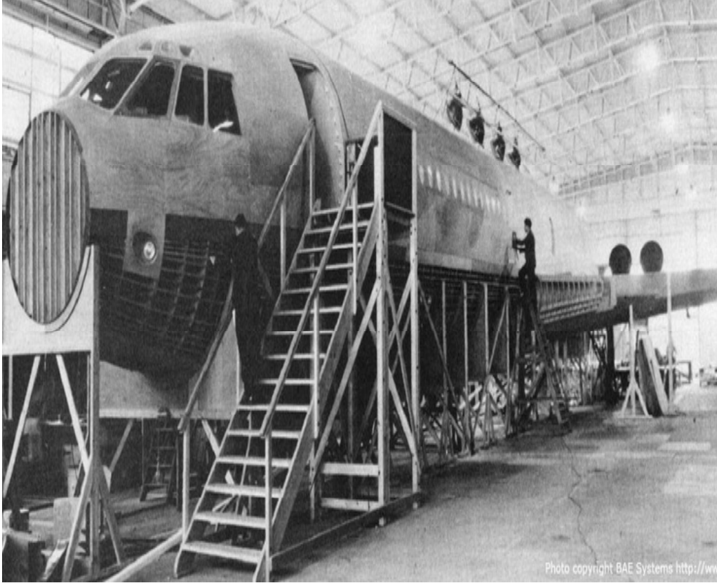
Figure 3.1: Assembly wooden mockup [6]
