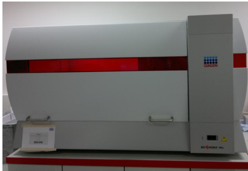
Figure 2.2: BioRobotMDa workstation employed for automated nucleic acid purification from salivary supernatant samples (Qiagen, UK) [source: Virology Unit at Barts and The London NHS Trust].
