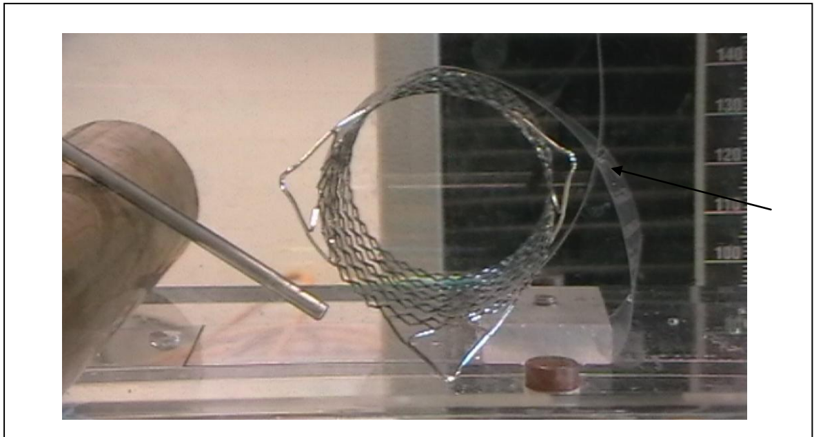
Figure 96 2G ATAG with sinus feelers within the constriction loop
