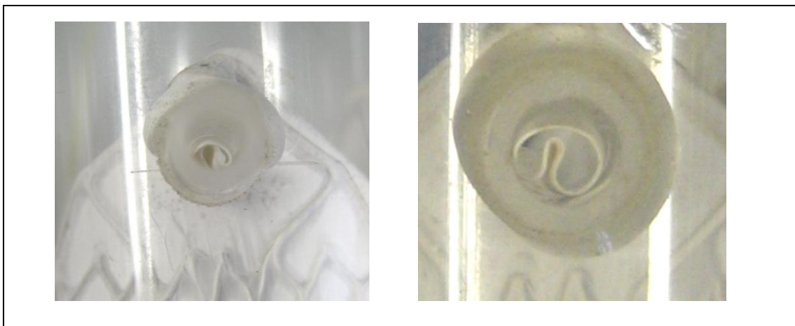
Figure 110 Involution and collapse of the PU materials within the coronary ostia
