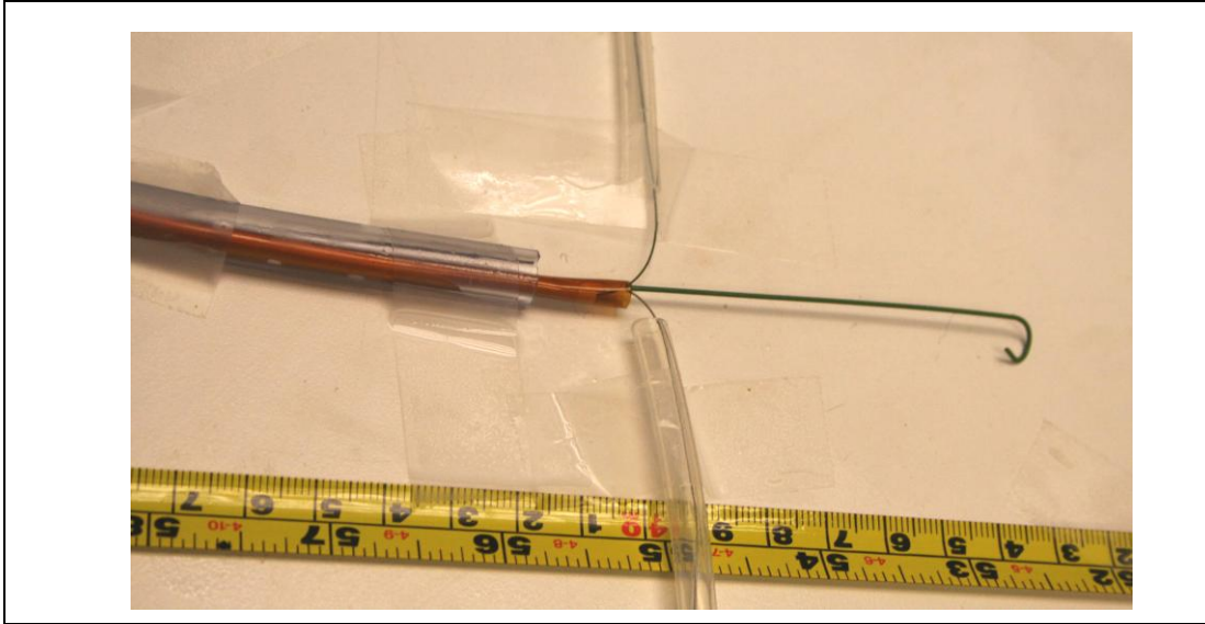
Figure A-5 Delivery catheter was advanced to the guide wire crossing location
