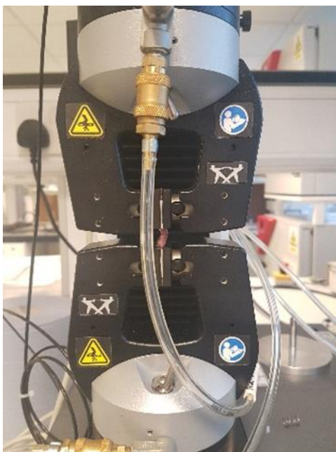
Figure 61: Uniaxial Rig Set-Up . Tissue sandwiched between four pieces of sand paper and gripped within the uniaxial rig.
