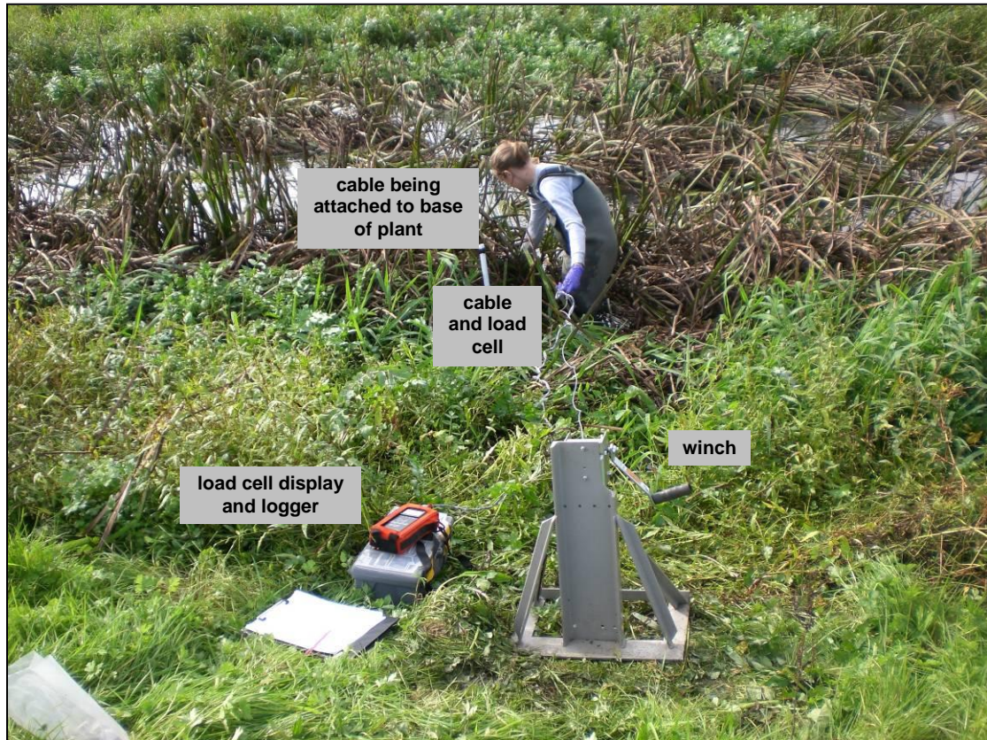
Figure 5.7: The plant pulling device installed in the field.
