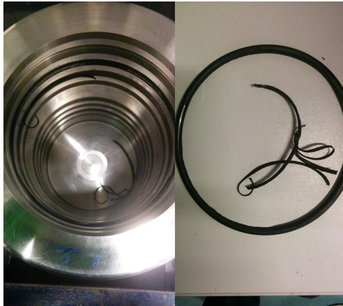
Figure 4.21: Nitrile O-ring used for the experiment plotted in Fig 4.20. The figure on the left shows the bottom of the sleeve with the shavings of the cleaved material. The figure on the right is the O-ring after the test with all the fractured material shown.
