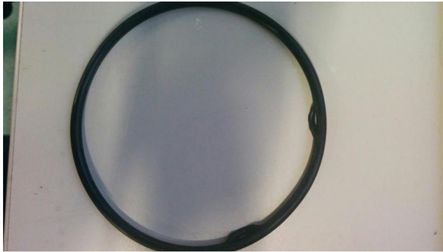
Figure 4.23: Nitrile O-ring used for the experiment lined out in Fig 4.22. The O-ring has clear signs of damage during insertion.
