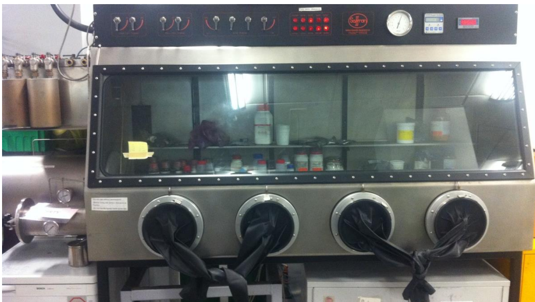
Figure 3.2: Saffron scientific glove box used for powder handling under inert environment
