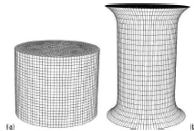
6 a meshed undeformed cylindrical component and b meshed cylindrical component deformed in tension
