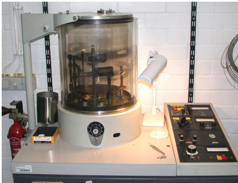
Fig. 24 Thermal Vacuum Evaporator (Edwards Coating System E306A, Crawley, UK)
