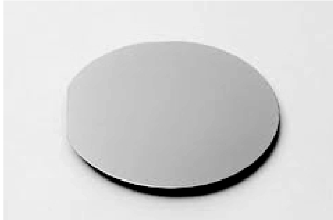
Fig. 22 P-type silicon wafer with a diameter of 15 mm, purchased from Si-Mat, Germany
