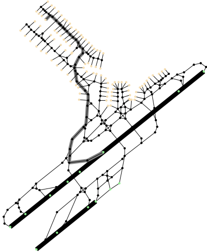
Fig. 2. Example of a generated airport taxiway network. Yellow, black, and green notes are gates, taxiways, and runways, taxiways. The ground movement route in gray is map matching result from the runway to the gate.
