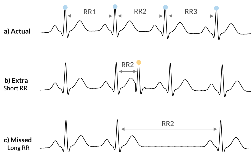
Figure 2.3: A schematic diagram of ECG signals a) without artefacts, b) with an extra beat, and c) with a missed beat.
