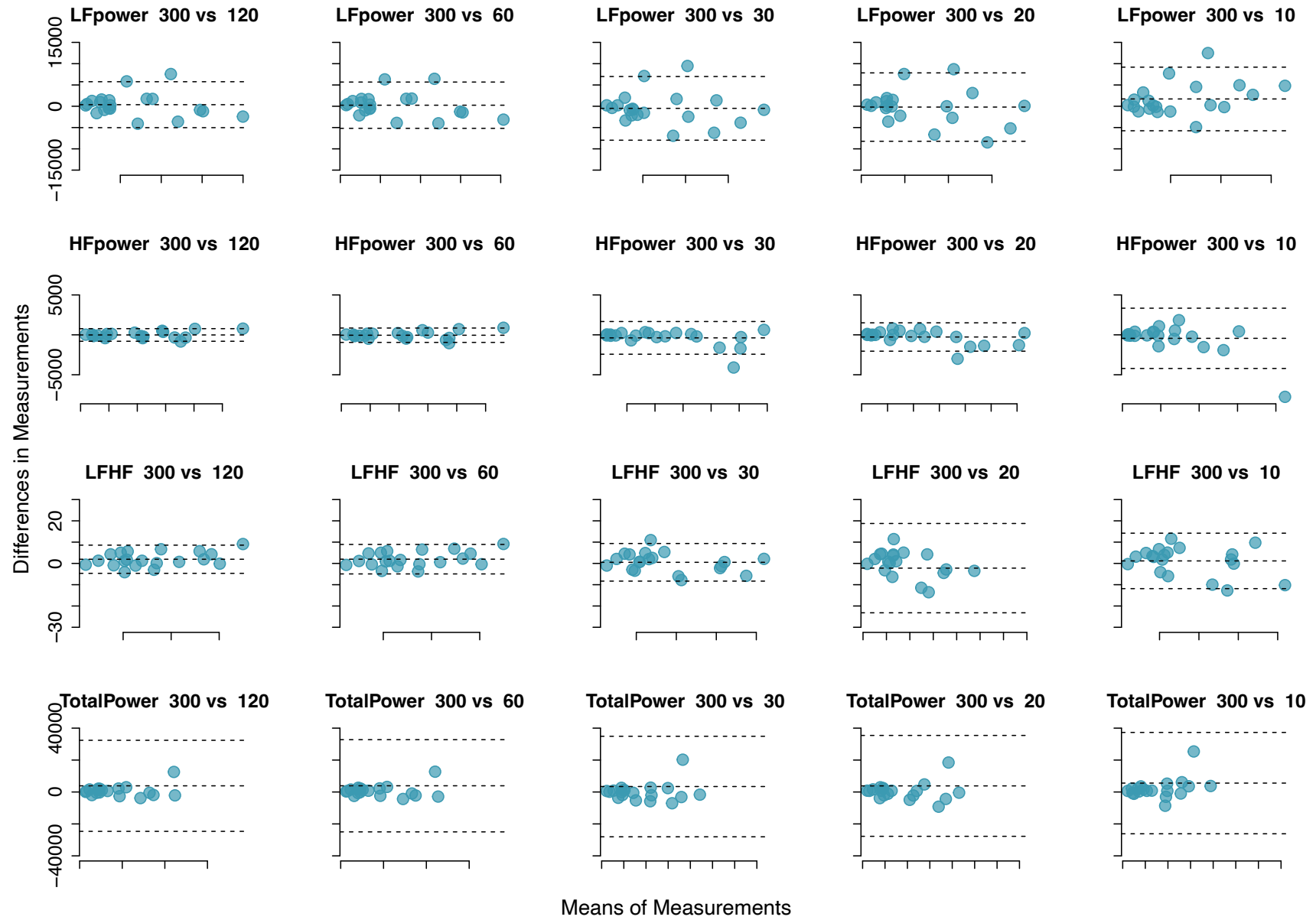
Figure D.8: Bland-Altman Plots with 95% Limits of Agreements of HRV Frequency-Domain Measures during Paced Breathing.
