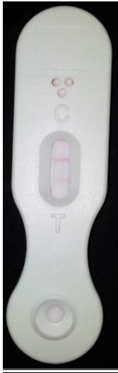
Figure 8. Antibody-based detection of Aspergillus antigen.
