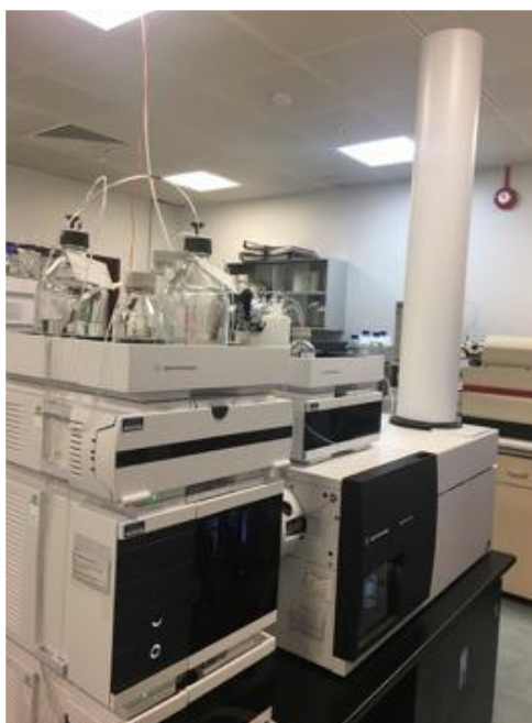
Figure 28: Agilent Technologies 1290 Infinity II – 6545 Q-TOF LC/MS instrument with electrospray ionization in positive ion mode
