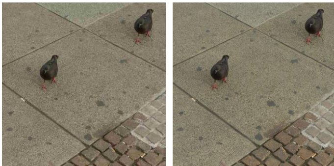
a) JPEG compression: left - quality factor: 20, name: "015_F_JC1.jpg", right - quality factor:80, name: "015_F_JC7.jpg"
