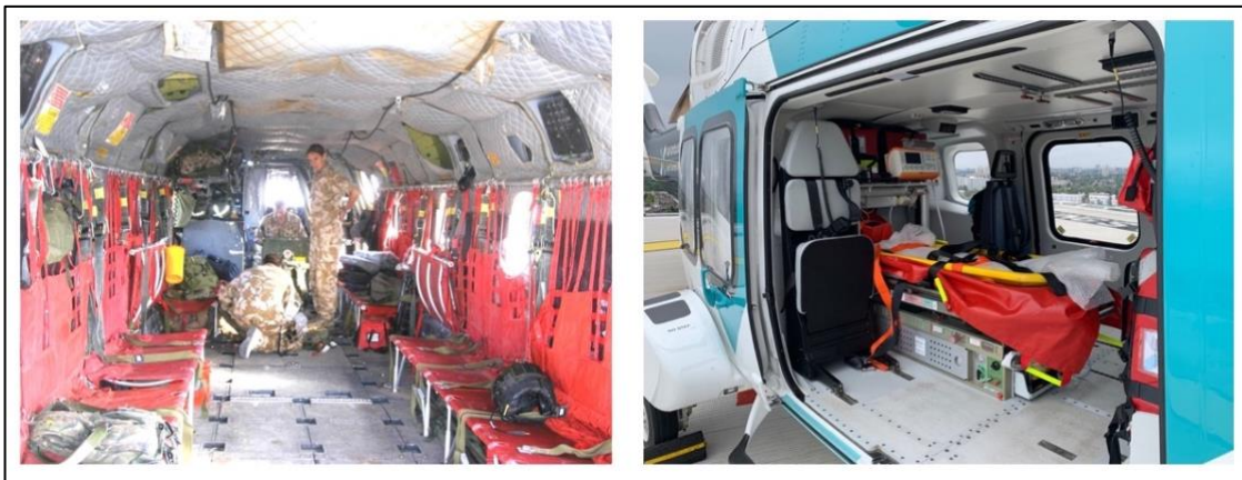
Figure 3: Comparison of the space to provide medical care in two medically fitted helicopters. Left: Military; inside the Chinook (CH47), photograph from Greaves 26 , Right: Civilian; inside the AW169 helicopter used by Air Ambulance Kent, Surrey and Sussex photograph authors' own
