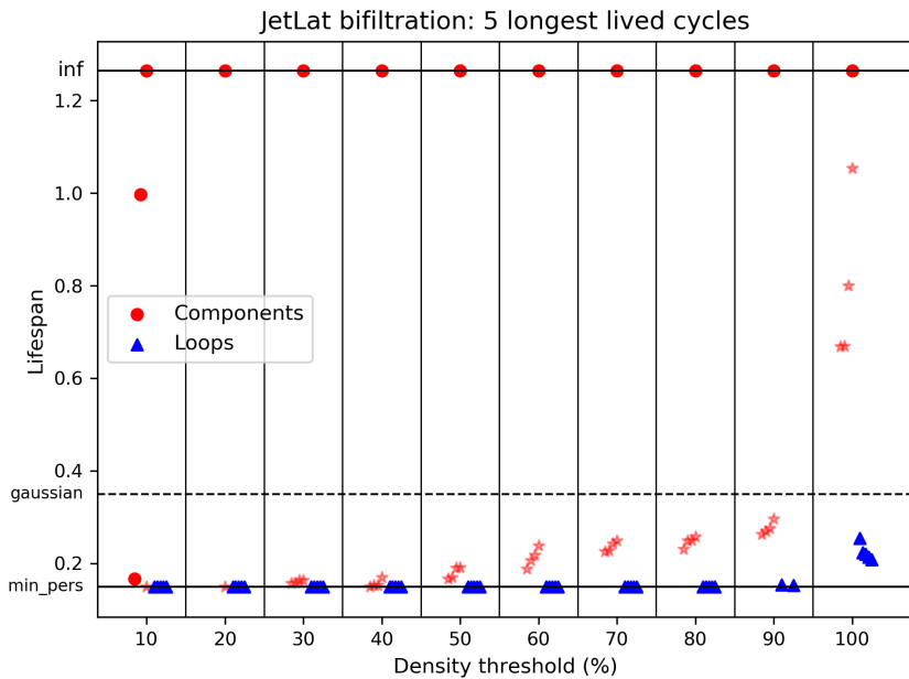
Fig. 21 A distance-density bifiltration of the JetLat data set. For each density threshold on the x -axis, the lifespan of the 5 longest-lived connected components (red dots if the component contains more than 3 points; red stars otherwise) and 5 longest-lived loops (blue triangles) are plotted. The stippled line shows the largest lifespan expected from Gaussian noise. The meaning of the min_pers parameter is explained in Section 4.2.
