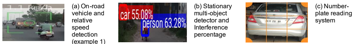
Figure 3: Image processing system in the proposed traffic monitoring system (with a maximum vehicle to drone distance of 15 meters).
