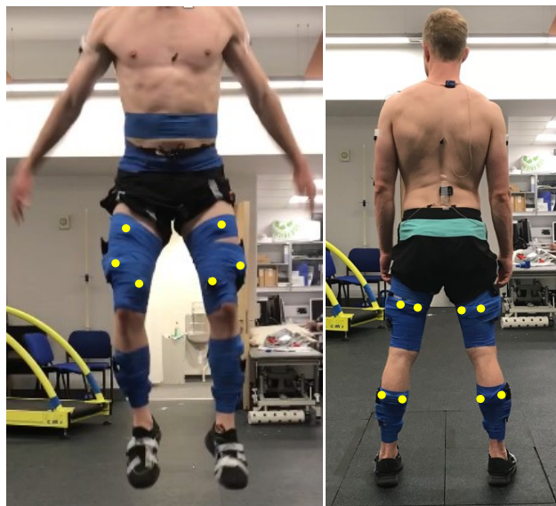
Figure 24: Lab protocol. Kinetics, kinematics, and stick figure configuration of the body. Basic foot (heel, first and fifth metatarsal), shank, thigh, pelvis (anterior and posterior superior iliac spine), trunk (xiphoid and T8 vertebrae), and arm (acromion and lateral epicondyle) markers were used. EMG sensors placements for both legs (yellow points). Keys: M, markers; R, right; L, left; MT, metatarsal; ASIS, anterior superior iliac spine; PSIS, posterior superior iliac spine; IC, iliac crista; AC, acromion; HLE, humerus lateral epicondyle; X, xiphoid; T8, T8 vertebrae; C7, C7 vertebrae; SJN, sternum jugular notch; MM, medial malleolus; LM, lateral malleolus; MFE, medial femoral epicondyle; LFE, lateral femoral epicondyle
