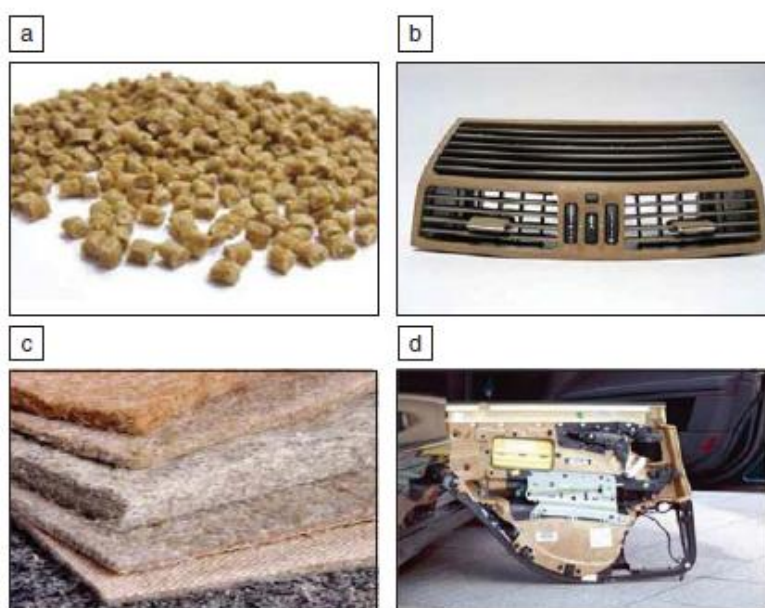
Figure 2.11. Examples of industrial biocomposite material forms and applications. (a) Thermoplastic/natural fibre granules for injection moulding; (b) section of a dashboard panel; (c) fibre mats for press-moulding; and (d) a BMW door panel. Images courtesy of Nova-Institute, Germany 44 .
