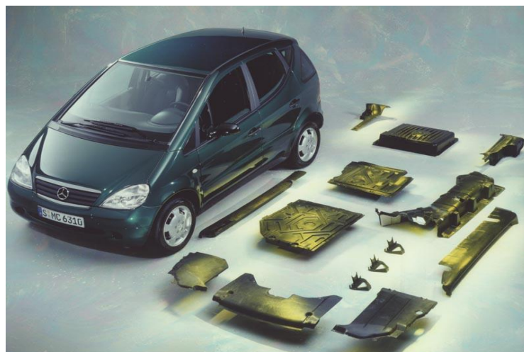
Figure 1.1. Elements of a Mercedes-Benz A-class car made with flax fibre mat reinforced polypropylene.
