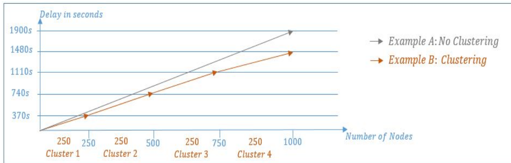
Figure 3.6: Transmission Delay in Typical LoRaWAN (example A) Vs. Proposed K-Means Clustering based Simple Transmission Priority Scheduling Technique (example B)
