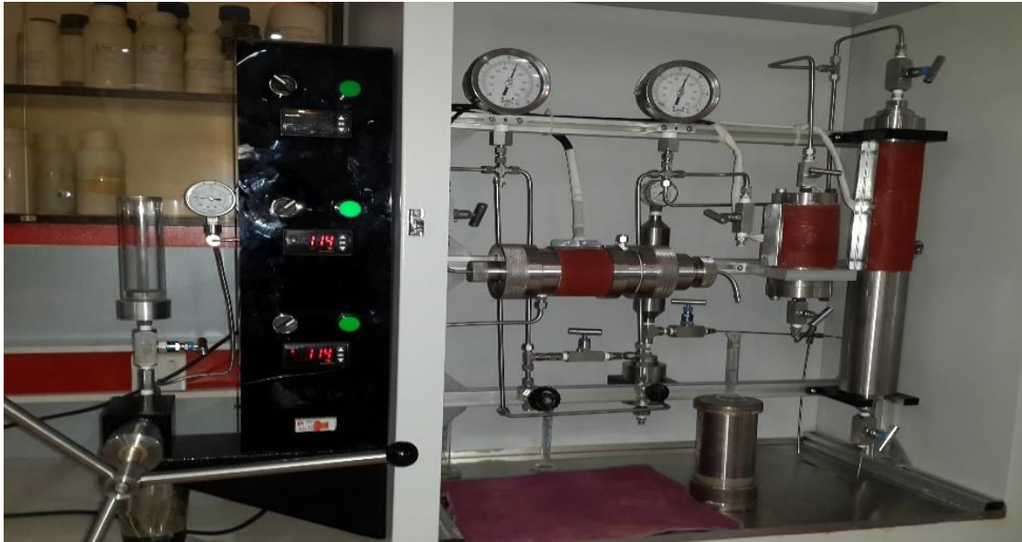
Fig 1. Customized Core Flood Unit for Drilling Fluid Formation Damage Measurement and Removal
