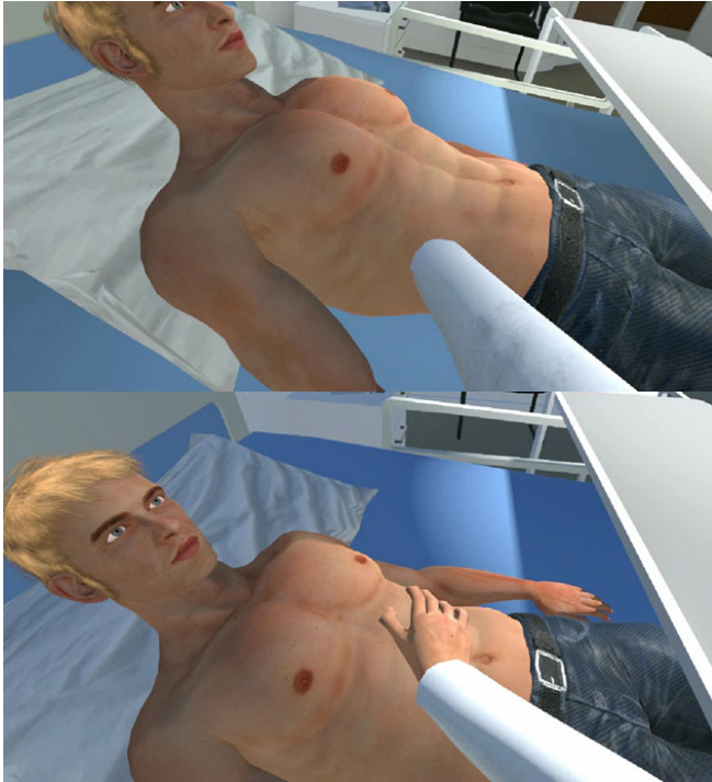
Figure 5. (Up) The user tries to palpate the patient, but there are no colliders enabled, so the hand goes through the virtual patient. (Down) The user tries to palpate the patient, but the colliders stop the hands from going through the virtual patient.
