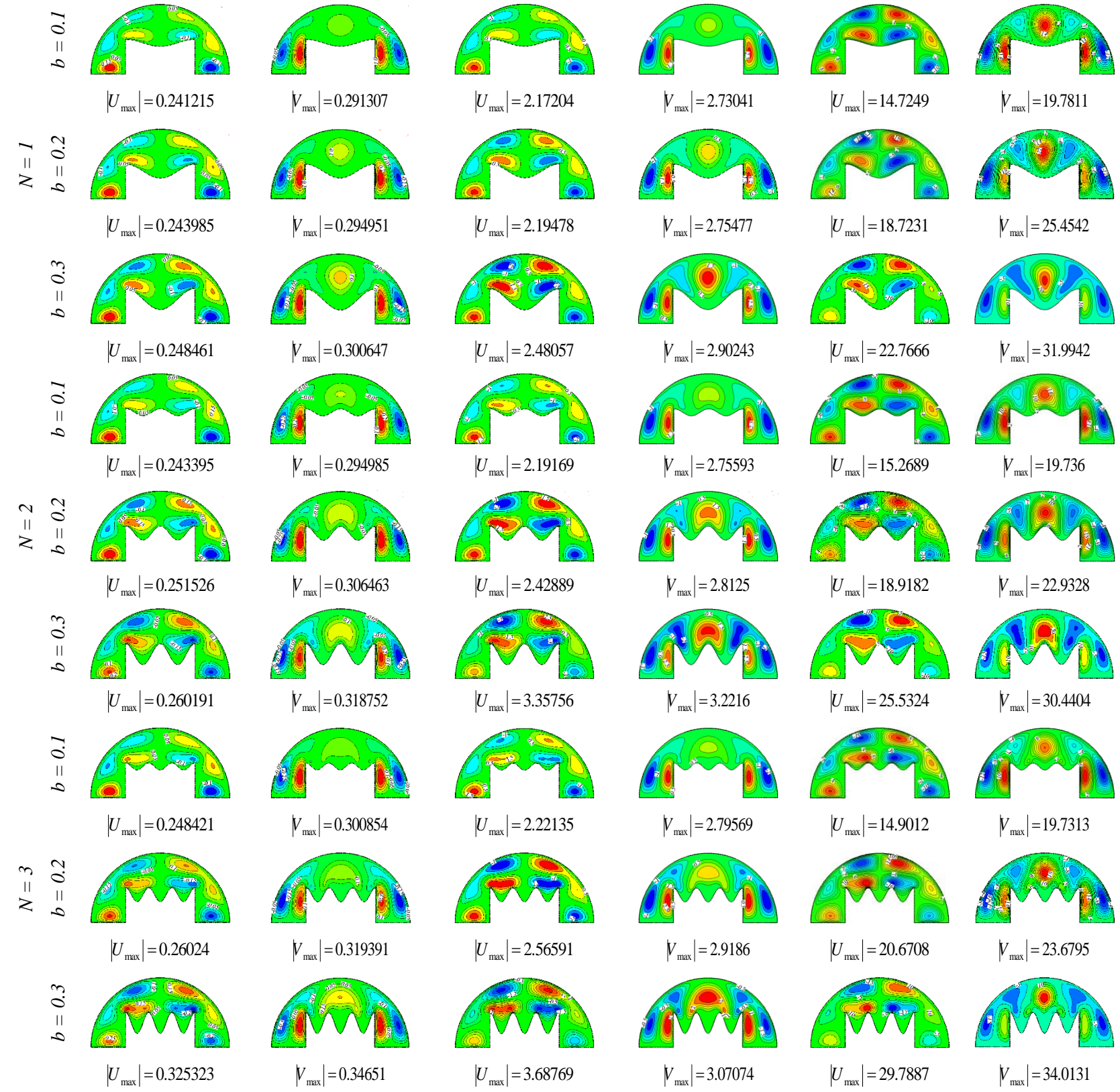
Fig. 8. U and V for varied measure of N, b, and Ra when H_s=1 , Da=10^{-1} , \phi=0.05 , Ste=0.313 , and \theta_f=0.2
