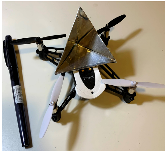
Figure 6: Parrot Mambo Minidrone, with a trihedral retro-reflector for the RCS, for increased RF detectability.
