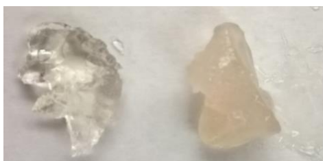
Figure 5. Image of CMC gels with a low (20:1) CMC: CaCl 2 ratio (left) and a high (1:1) ratio (right). It is clear that at high electrolyte concentrations CMC gels are more heterogenous and chains start to precipitate, with increased opacity of the corresponding materials.
