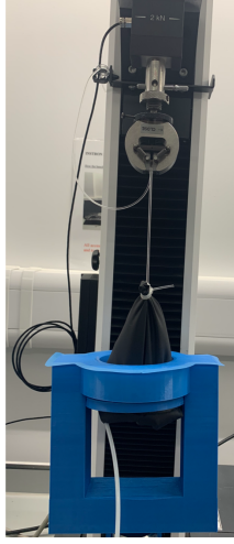
Fig. 5: Inhomogeneous eversion actuator mounted on a universal testing machine (UTM) for characterizing the generated forces
