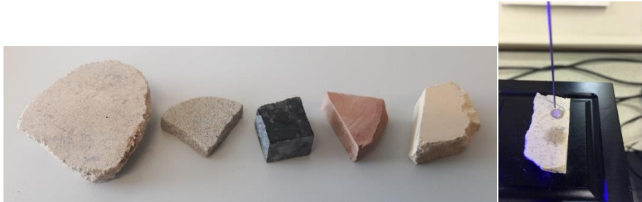
Fig. 2 The polished rock surfaces for contact angle measurement.
