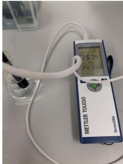
Conductivity measurement of surfactant solution.
