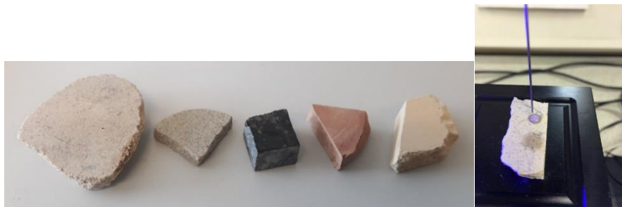
Fig. 2 The polished rock surfaces for contact angle measurement.
