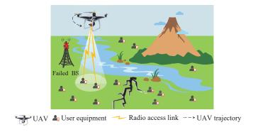
Fig. 1: UAV emergency communication networks.
