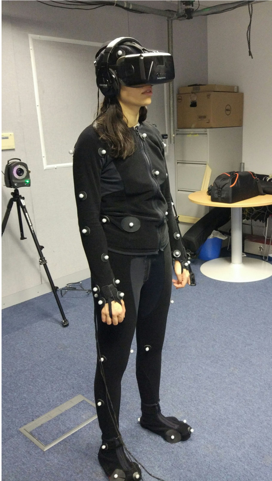
Figure 4.3: Participant wore black suits attached with markers and Oculus Rift DK2 (HMD)
