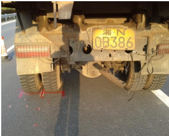
Figure 5 Loading using standard vehicles
