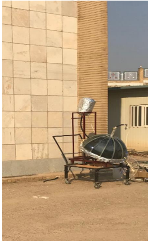
Figure 2 Photo of the hemispherical solar collector during an experimental run.
